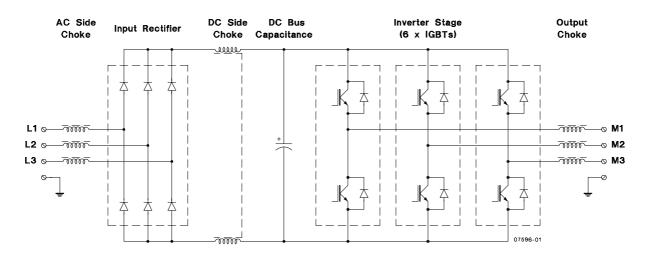
**Figure 1:** Power circuit of a Variable Speed Drive Inverter showing the DC-side choke, DC bus capacitor, input rectifier and inverter output stage and AC-side input and output chokes.
