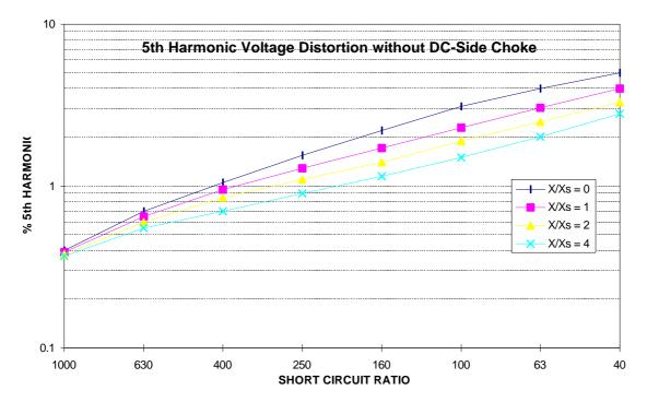
**Figure 2(c):** Percentage of 5 th harmonic voltage distortion for a typical variable speed drive <u>without</u> a DC-side choke. The effect of AC-side chokes (reactance X) are also shown for various sizes of X. Xs is the supply reactance.
