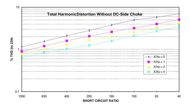
**Figure 2(d):** Percentage of total harmonic voltage distortion for a typical variable speed drive <u>without</u> a DC-side choke. The effect of AC-side chokes (reactance X) are also shown for various sizes of X. Xs is the supply reactance.
