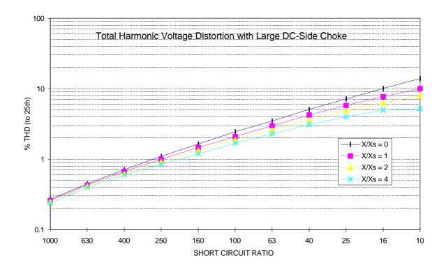
**Figure 2(b):** Percentage of total harmonic voltage distortion for a typical variable speed drive <u>with</u> a large DC-side choke. The effect of AC-side chokes (reactance X) are also shown for various sizes of X. Xs is the supply reactance.
