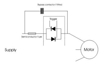
Semiconductor fuses are installed on the line side of the softstarter. The fuses must not be installed in the bypass circuit.
