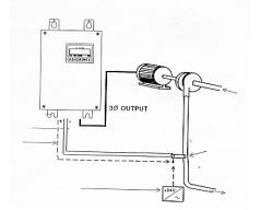
Refer to the instruction manual for comprehensive details on installation, in particular using screened motor cables.
