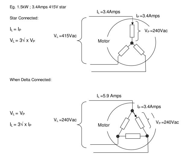
Therefore, the Line current or Full Load Current of the motor when connected in 240V Delta is **5.9Amps**. A Variable Speed Drive capable of a continuous output of 5.9 Amps is required.
