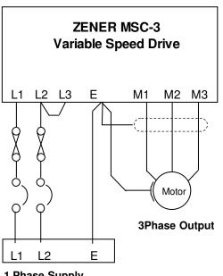
Speed control can be manually using the controls provided or remote speed potentiometer. A Pressure control system can be easily achieved using the drives internal PID control and an external pressure transducer.
